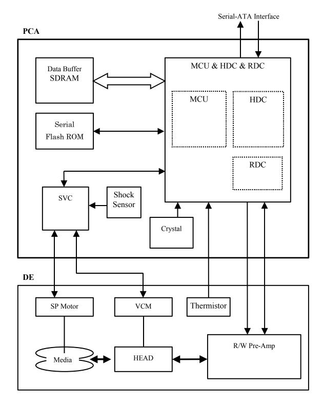
Figure 4.2 Circuit configuration
